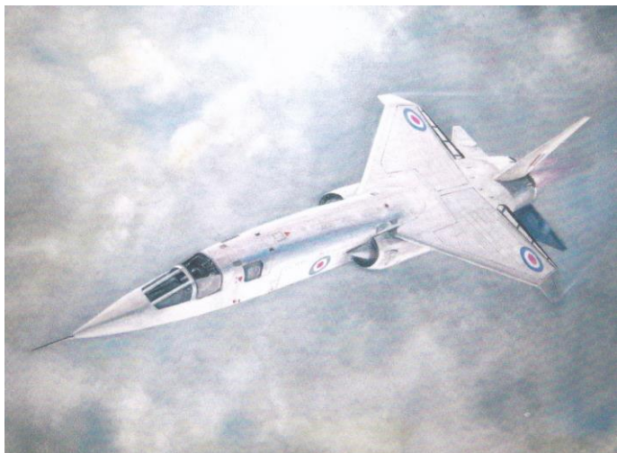
11 TSR2 (Tactical Strike and Reconnaissance – a misleading title!). The TSR2 was developed during the Cold War to deliver a nuclear weapon deep into Eastern Europe. It was intended to fly below enemy radar, guided by a navigational system designed by Ferranti, Edinburgh. The project was scrapped in 1965. There was never a TSR1!
